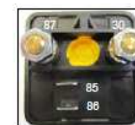
DETALLE RELE DE ARRANQUE 24V / STARTER RELAY 24V
