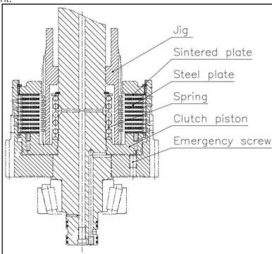
[Fig-10] Structure of clutch
