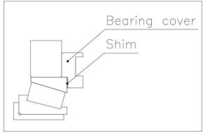
[Fig-13] Shim adjustment for pinions
