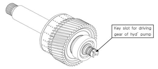
The astern shaft Ass'y consists of the same parts as the input shaft Ass'y except for the astern shaft sub Ass'y and pump driving block at the rear of shaft.
