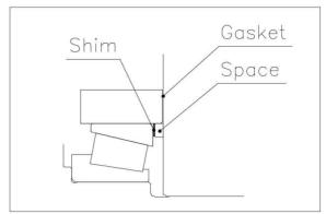
[Fig-15] Shim adjustment for astern shaft
