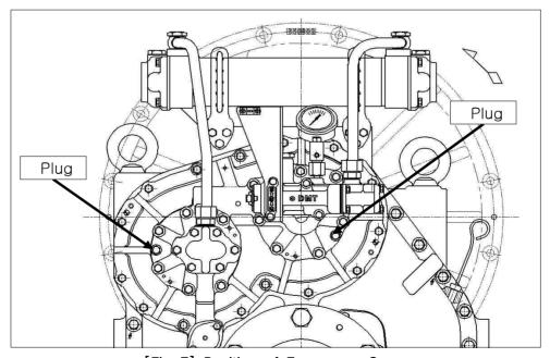
[Fig-7] Position of Emergency Screw
