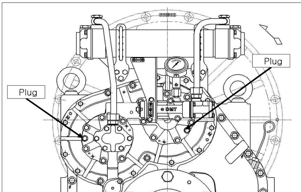
[Fig-7] Position of Emergency Screw
