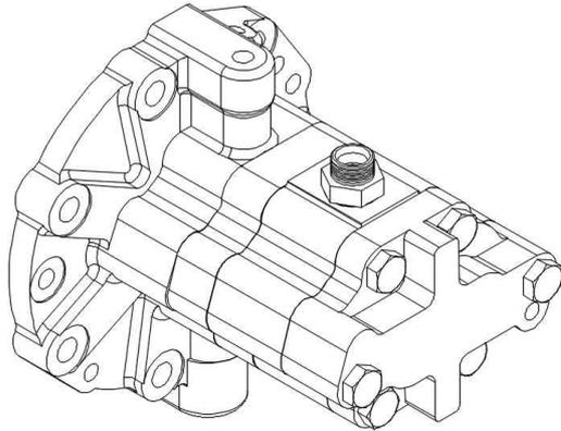
The pump holder is made of cast iron. The hydraulic pump is the circumscribed gear type, and bolted on the pump holder. The pump driving gear is driving block and spline fitted at the end of the astern shaft, and rotated at the same speed as that of engine, but in the opposite to engine direction.
