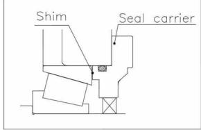
[Fig-12] Shim adjustment for output shaft
