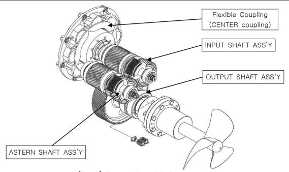
[Fig-1] Construction of Marine transmission
