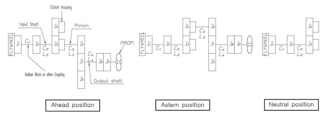
[Fig-3] Sequence of power transmission
