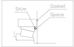
[Fig-14] Shim adjustment for input shaft
