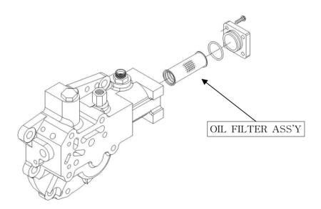
It is assembled to valve holder Ass'y and re-filters the oil which is filtered by the screen filter on the pump inlet' side. Afterwards the oil is sent to valve. it has the stucture to easily be cleansed by disassembling only filter's cover.
