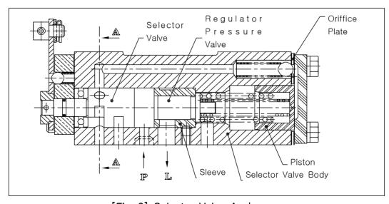
[Fig-6] Selector Valve Ass'y
