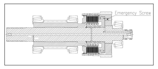
[Fig-8] Position of Emergency Screw
