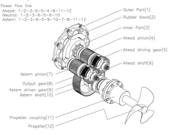
[Fig-2] Drive line system of marine Transmission
