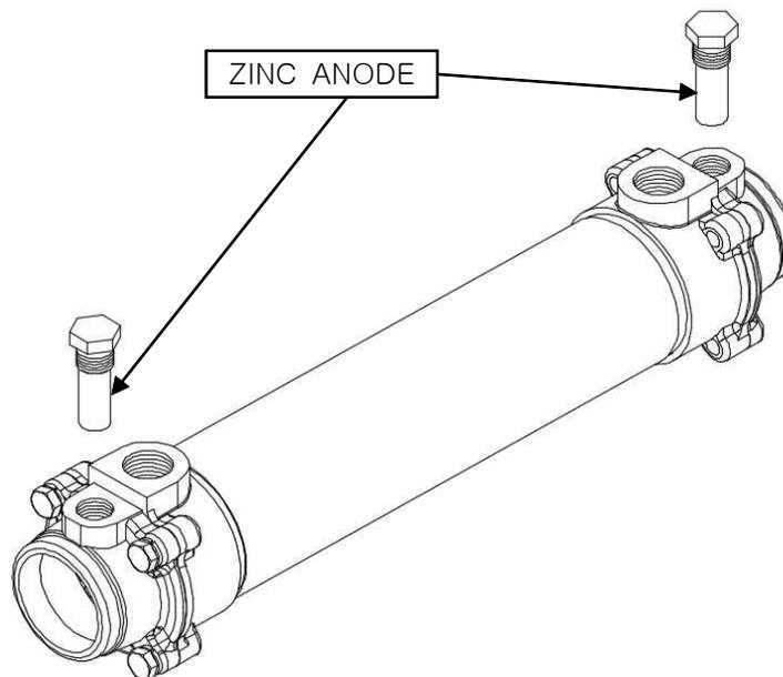
Oil Cooler is the device that cools the operating oil inside of marine gearbox and uses the seawater as cooling water. It is bolted on the cooler fixing block fitted in the case and cools the oil supplied from hydraulic pump and sends to the secondary oil filter. It uses Aluminum brass pipe which is strong against corrosion, and applies the Zinc anode.
