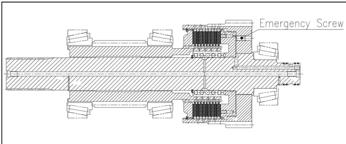
[Fig-8] Position of Emergency Screw
