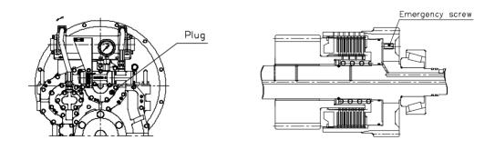
[Fig-7] Position of Emergency Screw
