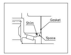
[Fig-10] Input and Astern Shafts
