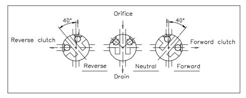
[Fig-5] Oil Passage of Selector Valve [SEC. A-A of Fig-6]
