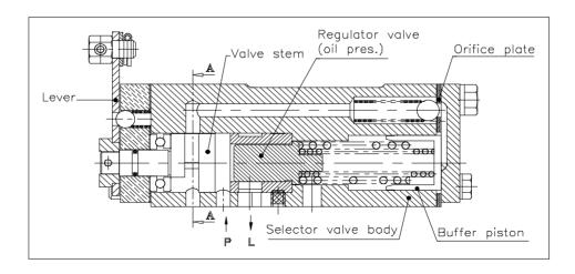
[Fig-6]Selector Valve Ass'y
