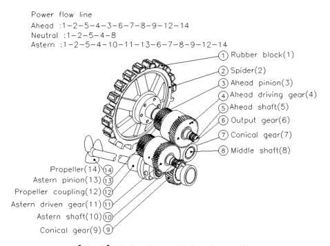
[Fig-2] Marine Transmission Power Flow
