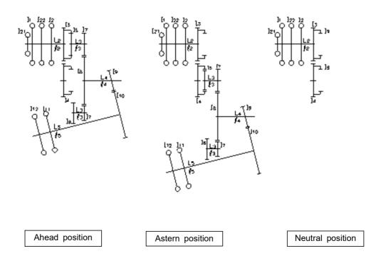
[Fig-3] Marine Transmission Power Flow
