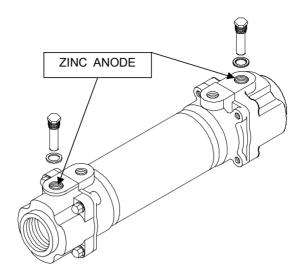
The oil Cooler is fixed above the case cover with bolts, and cools the oil supplied from the hydraulic pump before leading it into the secondary oil filter.
