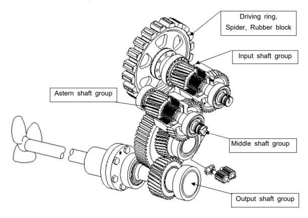
[Fig-1] Marine Transmission Construction
