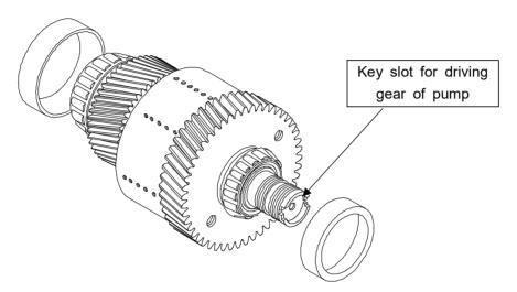
The astern shaft assembly has the same parts as those which the input shaft assembly has, except that the former has no spline in the front and has the hydraulic pump driving device in the rear end.
