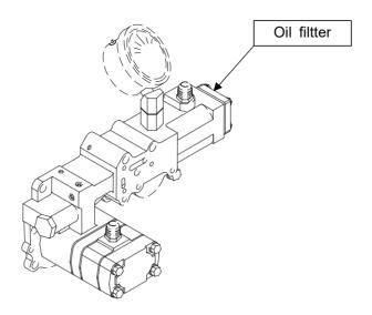
The manifold (valve holder) is made of cast iron, and includes oil pressure regulating valve.
