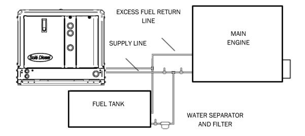
When it is connected to the fuel tank, a fuel filter must be installed. It is also good practice to install a tap in the supply line downstream of the tank, and a one-way valve (a non-return one only if the height difference is greater than 50 cm) to prevent the fuel system from being drained for any reason. Use a valve with an opening of 50 millibars. The fuel pipes must be made of hydrocarbon-resistant rubber, with an internal diameter of 6 mm.
